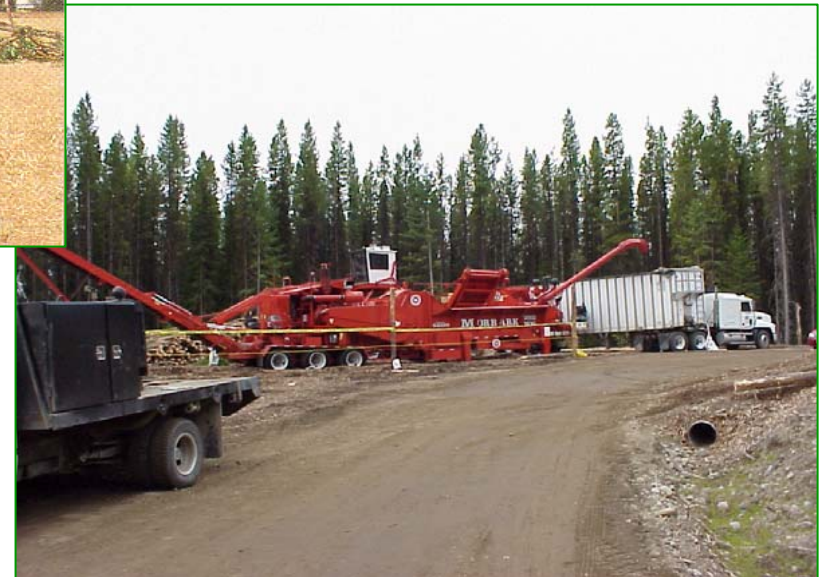
The DDC 5000-G whole-tree chipper is made by Peterson Pacific Corp.
