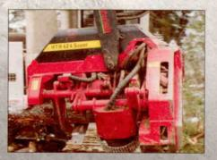
has a cutting capacity of 25.6-in. (65 cm) to process difficult, heavy-limbed or crooked stems into clean log lengths.
