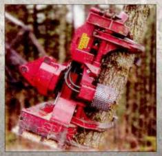
Quadco offers two purpose-built controlled falling and processing heads available in 22 and 24 in. cut designed for mounting on 22 ton or larger excavators or purpose-built feller bunchers. Accumulator arms provide multi-stem tree handling. Both heads feature a Motomit CANbus control system, high performance intermittent saw discs and .404 pitch top saws. Controlled mounts with float allow superior tree handling for harvesting and processing applications.
